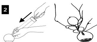
Insert the nozzle into the balloon, so that tip is in the center of the balloon. Hold it securely with one hand. Push water into balloon and continue to pump air into balloon until it is 3" (80 mm), the size of baseball. Wetting the balloon is better for insertion.
